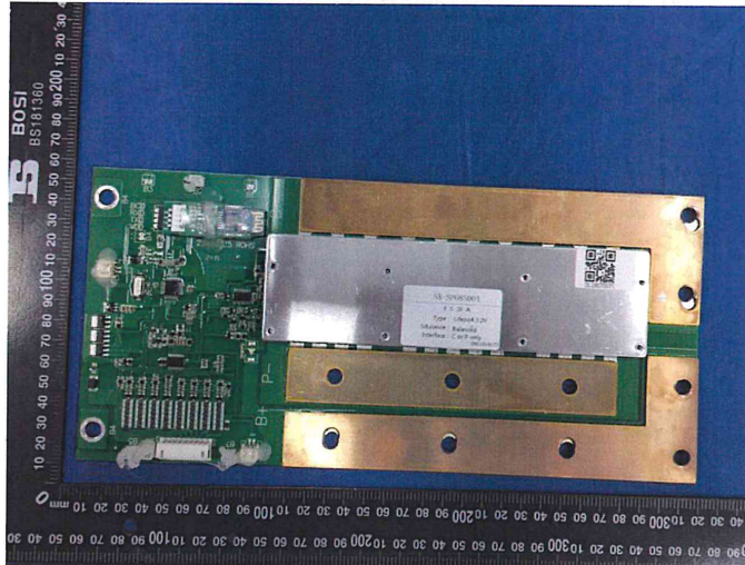
Picture 5. Protection board view
